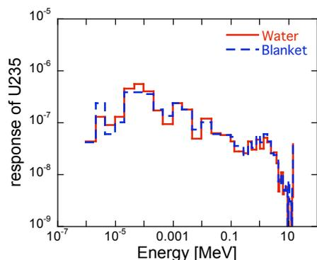
Fig.5 Energy dependence of the neutron response of a 1 mm cadmium-coated MFC in models in which a branch pipe is filled with (a) water or (b) materials used in the blanket module.
