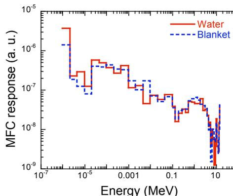
Fig.4 Energy dependence of MFC response to neutrons as they are affected by a branch pipe filled with (a) water or (b) materials used in the blanket modules.
