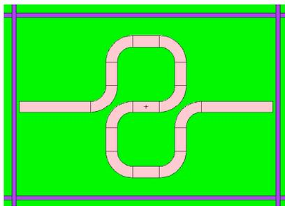
Fig.2 Image of the part of the branch pipe in the MCNP input file. Other shows the branch pipe and green shows the blanket module.
