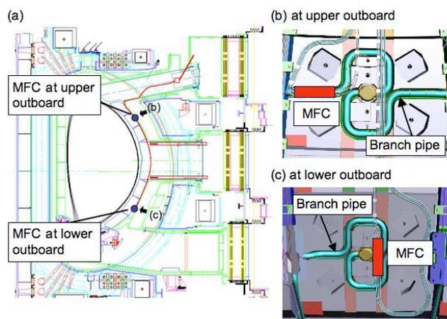
Fig.1 Location of MFCs on the ITER poloidal cross section (a) and schematic view of the installation position of MFCs at the upper outboard (b) and lower outboard (c) locations.
