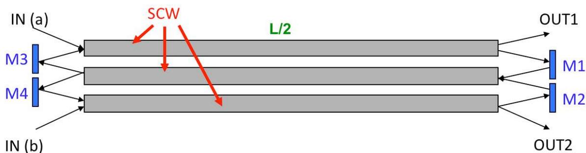
Figure 1: schematic view of the SCW diplexer-combiner
