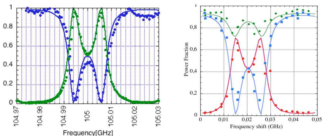
Figure 2: Power distribution in OUT 1 (blue) and OUT 2 (green/red) when power was launched in channel 1: test performed with the VNA (left) and with a quasi-optical bolometer (right).
