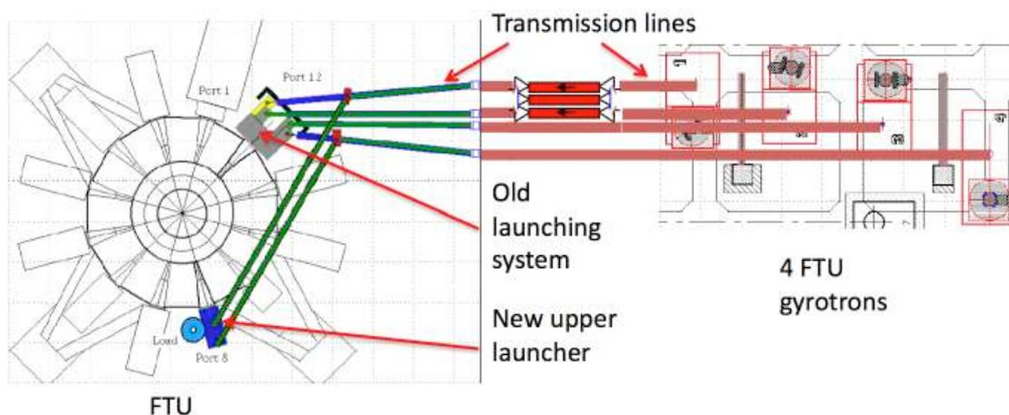
Figure 3: Overview of the old/new launching system of FTU.
