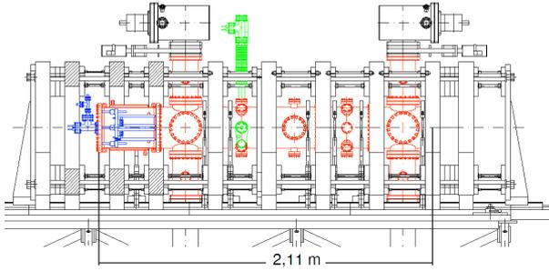
**Figure 2:** GyM design: in red the vacuum chamber, in blue the source and in green the electrostatic probes
