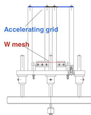
**Figure 3:** Hot filament source
