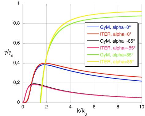
**Figure 6:** The imaginary part  $\gamma$  of the frequency versus the wavevector  $k$  for  $\alpha = \pm 85^\circ, 0^\circ$ , for typical GyM and ITER parameters.  $\gamma$  and  $k$  are normalized according to the rules discussed in [3].
