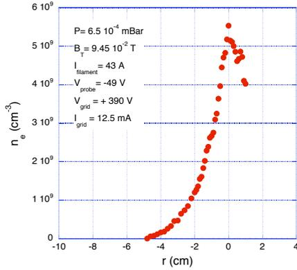
**Figure 4:** (left) Electron density profile from the ion saturation current, measured at 60 cm from the grid.
