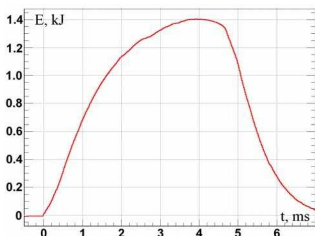
**Figure 1.** Time behavior of energy content of plasma in GDT during NB injection
