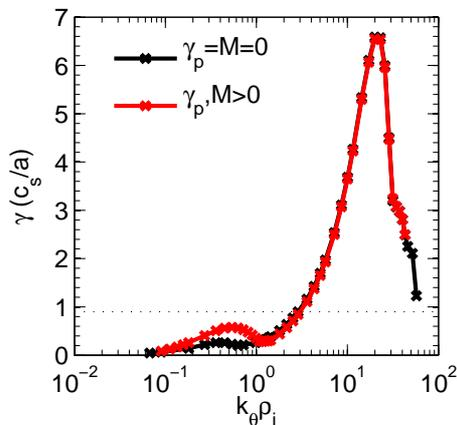
Fig. 4. Linear growth rates without (black) and with (red) finite toroidal flow and parallel flow shear.
