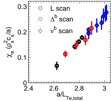
Fig. 2. Simulated transport  $\chi_e$  vs. net effective  $T_e$  gradient for various simulations.
