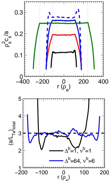
Fig. 1. (a) Profiles of  $\chi_e$  from local GYRO simulations with ExB shear (non-periodic BCs) using different box widths, boundary widths, and boundary damping strength. (b) Effective electron temperature gradient profiles (including time-averaged  $\langle \delta f_{n=0} \rangle_\theta$ ).
