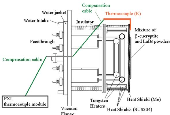
Fig. 1 Schematic of the plasma emitter
