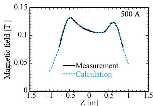
Fig. 5 A photo of the magnetic field coils (top) and measured and calculated profiles of magnetic field strength  $B_z$  (bottom).
