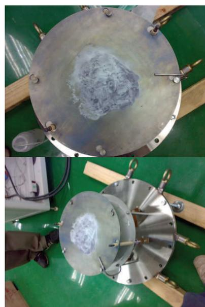
Fig. 2 Molybdenum plate coated with mixture of beta-eucryptite and  $\text{LaB}_6$  powders
