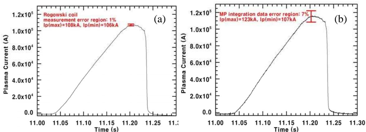
Fig. 1. (a) Plasma current measured by a RC.
