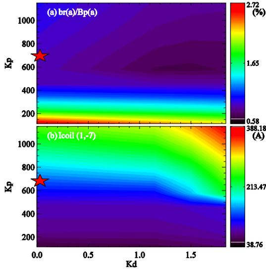
**Figure 3.** 2D scan of the normalized edge radial magnetic field (a) and the coil current requested by the feedback system (b) for the (1, -7) mode.
