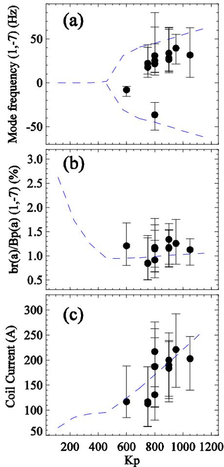
**Figure 2.** Effect of the proportional gain on the median of the mode rotation frequency (a), normalized radial amplitude (b), coil current (c) for the  $m = 1$ ,  $n = -7$  mode (error bars represent the 25<sup>th</sup> and the 75<sup>th</sup> percentile) estimated during the flat top of reproducible discharge at 1.4 MA. The blue curve represents the trend predicted by the model.
