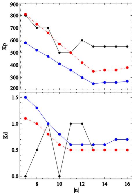
**Figure 4.** Values of  $K_p$  and  $K_d$  gains applied to TMs ( $m=1, n=-16,-7$ ). The black dots correspond to the empirical set, the blue dots, the optimal set suggested by the model, the red dots, the optimal experimental set.
