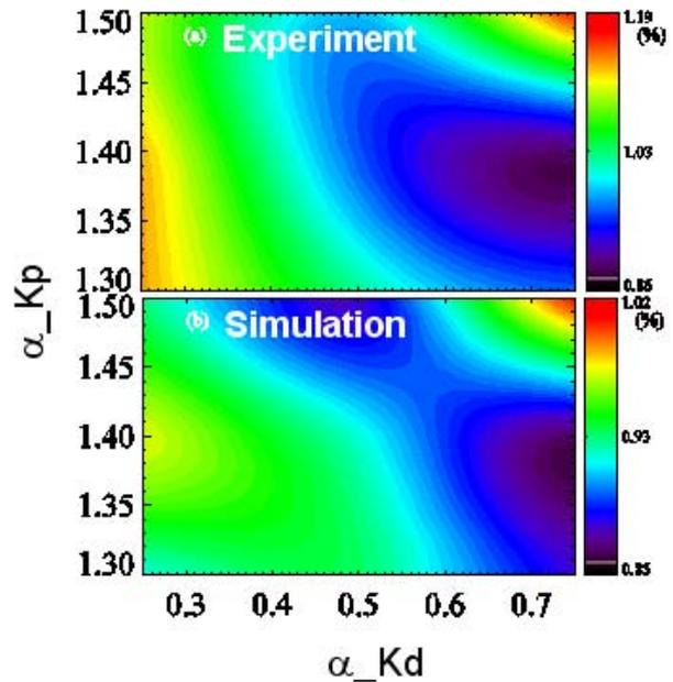
Figure 5. Experimental (a) and simulated (b) contour plot of the total radial magnetic field
