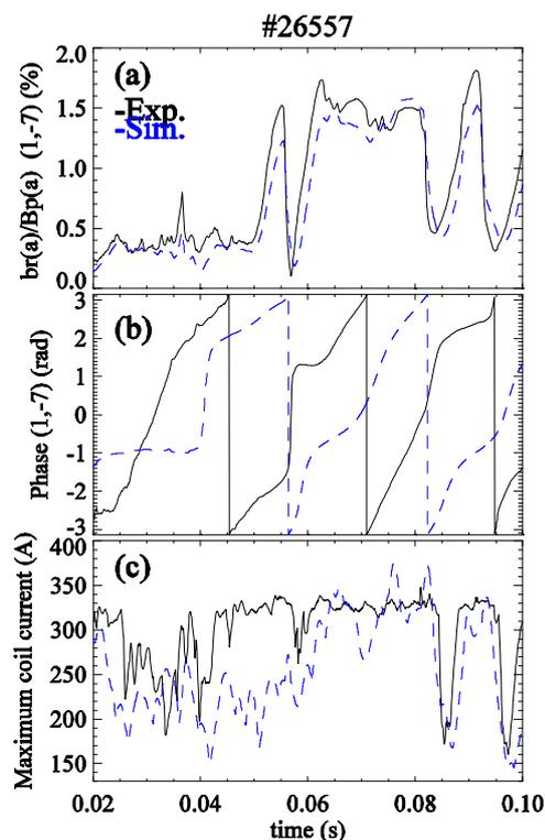
**Figure 1.** Normalized edge radial magnetic field (a), phase (b) of the (1,-7) mode and maximum coil current of the feedback system (c) in a 1.7 MA discharge and from the simulation.
