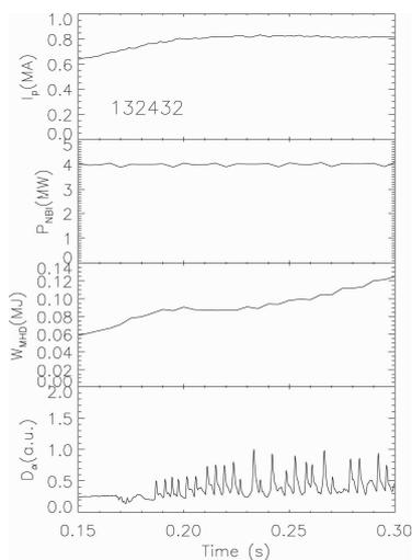
Fig. 3 Time trace of several plasma parameters for the same time window shown in Fig. 2. Note the increase of plasma stored energy ( $W_{MHD}$ ), which is reflected by the increase of peak temperature and heat flux at the ELM peaks in Fig. 2
