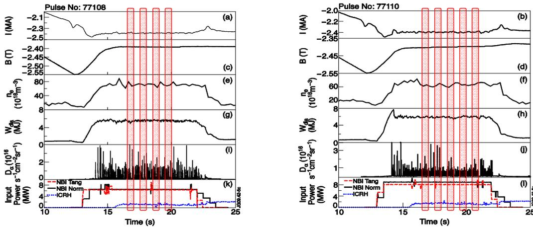
**Figure 1:** Time traces of plasma current a)-b), magnetic field c)-d), volume averaged electron density e)-f), diamagnetic energy g)-h), outer divertor  $D_\alpha$  i)-j) and additional heating power k)-l) for pulses 77108 and 77110.
