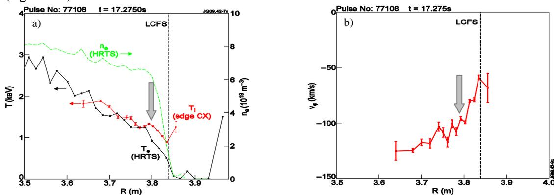
**Figure 2:** Profile of ion temperature (—) given by edge CXRS, electron temperature (—) and density (—) given by HRTS (a) and toroidal velocity profile given by edge CXRS (b) for JET pulse no 77108 at  $t = 17.275\text{s}$ .
