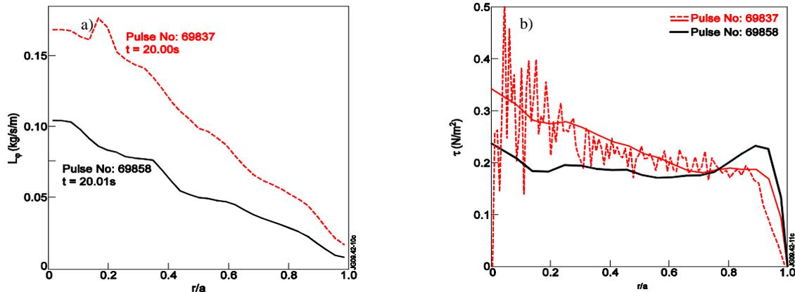
**Figure 4:** (a) Angular momentum density profiles for pulse 69858 (—) and 69837 (—). (b) torque profile calculated by PENCIL, for pulse 69858 (—) and 69837 (—), and calculated by ASCOT for the latter (---).
