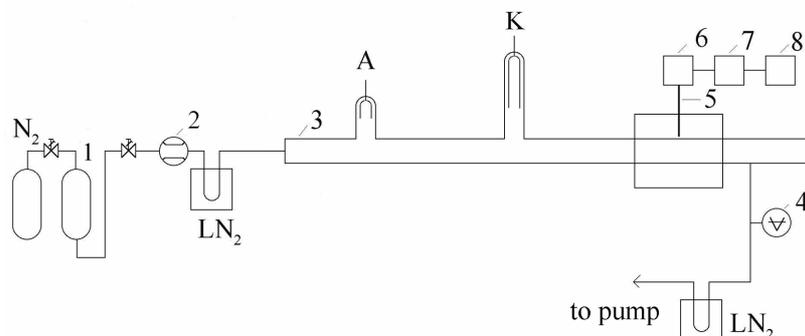
Fig. 1 Scheme of the experimental set up. 1 – catalyzer Oxiclear; 2 – mass flow controller; 3 – Pyrex discharge tube; 4 – capacitance gauge; 5 – quartz optical fiber; 6 – monochromator Jobin Yvon Triax 550; 7 – CCD; 8 – PC.
