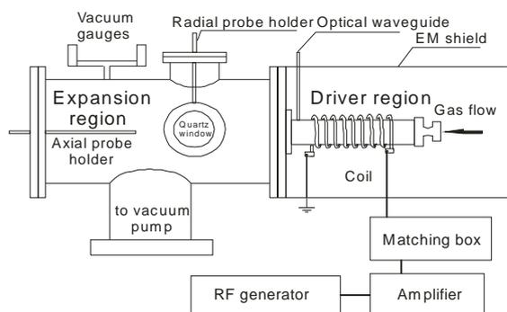
**Fig 1.** Scheme of the experimental set-up.
