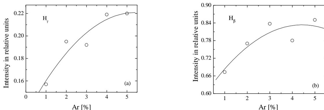
**Fig. 3.** Influence of argon percentage on the maximum intensities of the Balmer line  $H_\gamma$  in (a) and  $H_\beta$  in (b).
