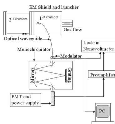
**Fig 2.** Arrangement for the optical emission spectroscopy diagnostics.
