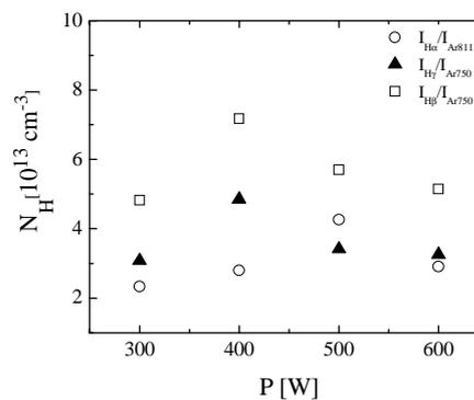
**Fig. 5.** Variation of the hydrogen atom density with the applied power.
