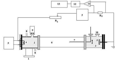
Figure 1: Sketch of experimental setup to record discharge current fluctuations in the tube filling by Helium gas. The scheme of the measurement setup and the experimental discharge tube, 1) to vacuum pumps, 2) copper cylinder, 3) power supply 4) hot cathode, 5) anode plate, 6) glass tube, 7) single Langmuir probe, 8) water cooling, 9) Pirani pressure gage, 10) gas inlet, 11) OP – Amp, 12) low pass filter, 13) A/D card and PC.
