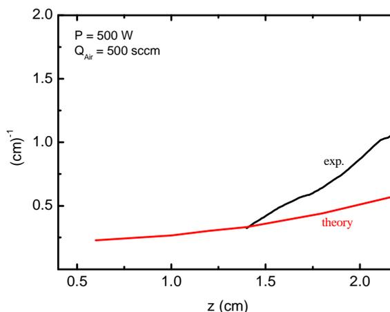
Fig. 8. Attenuation coefficient axial dependence
