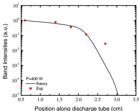
Fig. 7. Axial dependence of the intensity of NO( ) band radiation. Points – experiment; curve – model calculations (1% water vapour).
