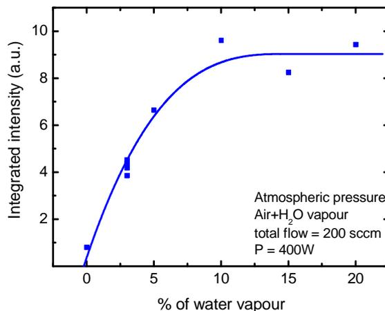
Fig. 6. OH integral intensity vs. percentage of water vapour.
