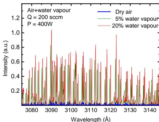
Fig. 2. OH spectra for three different percentages of water vapour.
