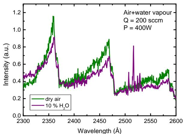
Fig. 5  $\text{NO}(\gamma)$  spectra for different percentages of water vapour.
