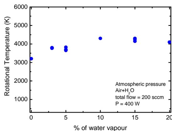
Fig. 4. Gas temperature vs the percentage of water vapour.
