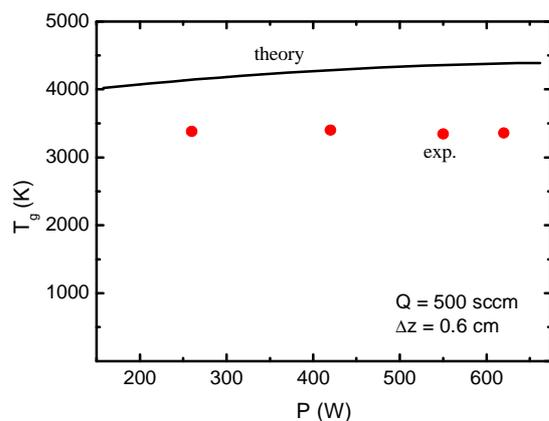
Fig.3. Dependence of the gas temperature on the microwave power delivered to the launcher (1% water vapour).
