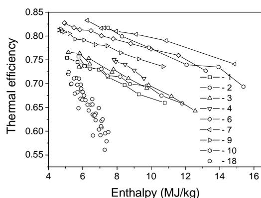
Figure 2. Thermal efficiency of plasma torch versus enthalpy of plasma jet.  $L/d$ : 1 – 23/6; 2 – 27/6; 3 – 34/7; 4 – 34/8. Items 5 – 8 the same as 1 – 4, but different impedance of power supply; 9 – plasma torch PDS-3.
