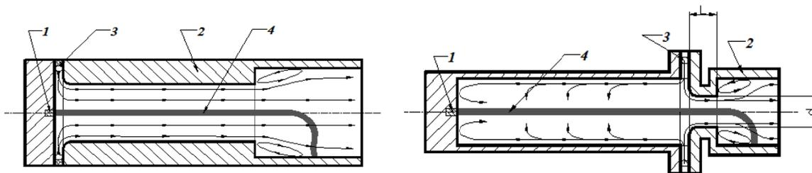
Figure 1. Scheme of the traditional plasma torch (to the left) and one with reverse vortex (to the right). The flow lines of gas are sketched. Radial distributions of pressure  $\Delta P = P - P_0$  ( $P_0 = 1$  atm) are shown at the bottom of the scheme. 1 – thermionic cathode; 2 – anode; 3 – vortex chamber; 4 – electric arc.
