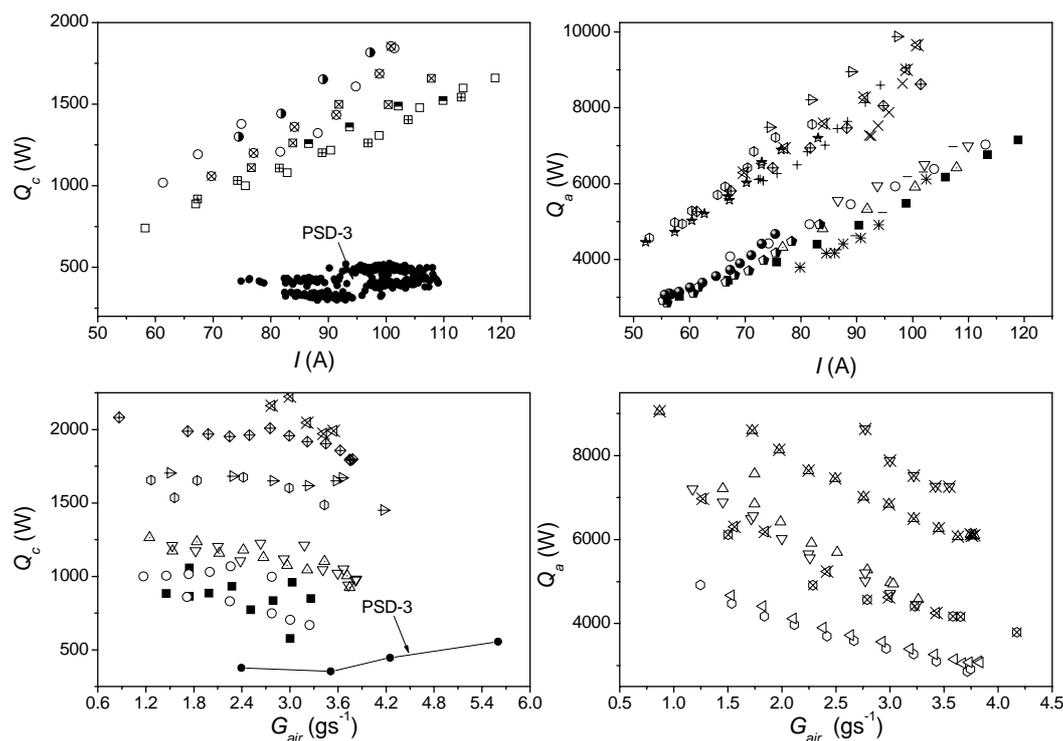
Figure 4. Thermal characteristics of plasma torch with reverse vortex for different configuration of diaphragm and working conditions.
