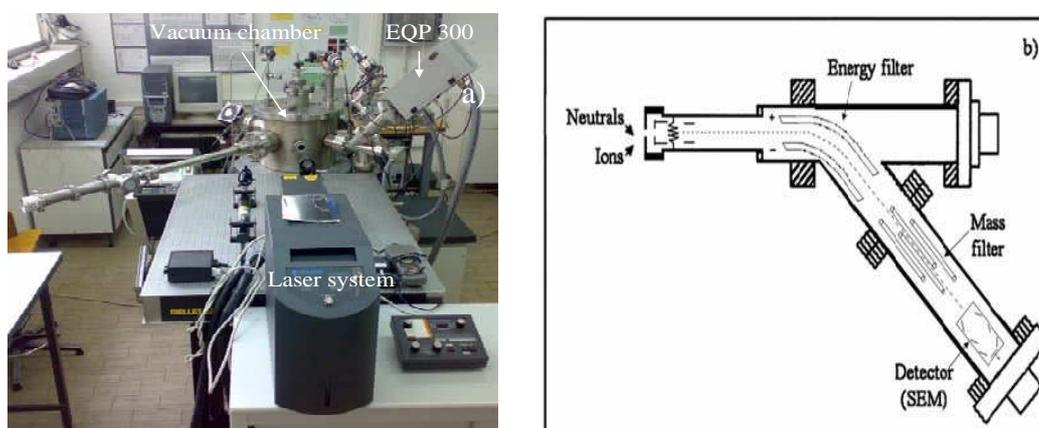
**Fig. 1:** Photo of the experimental setup (a) and scheme of the EQP instrument (b).
