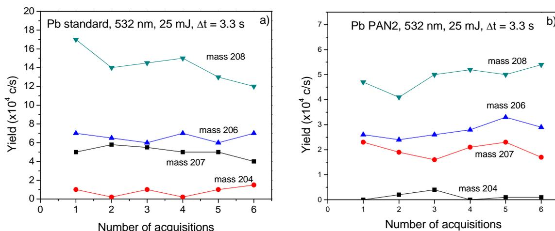
**Fig. 2:** Mass yield as a function of the acquisition number for four isotopes of the lead and for the standard (a) and PAN 2 (b) irradiation.
