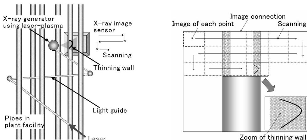
Fig. 1 (a) Concept of radiographic testing in a very narrow space and (b) for wide regional diagnosis.
