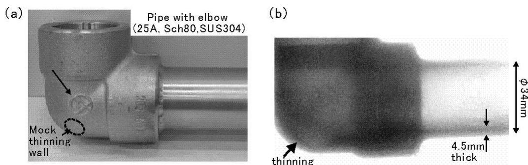
Fig. 5 (a) Photograph of a sample object and (b) the x-ray image obtained laser-plasma x-ray.
