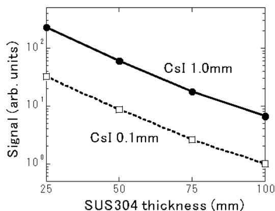
Fig. 4 Comparison of sensor signal between 0.1 mm and 1 mm thick CsI.
