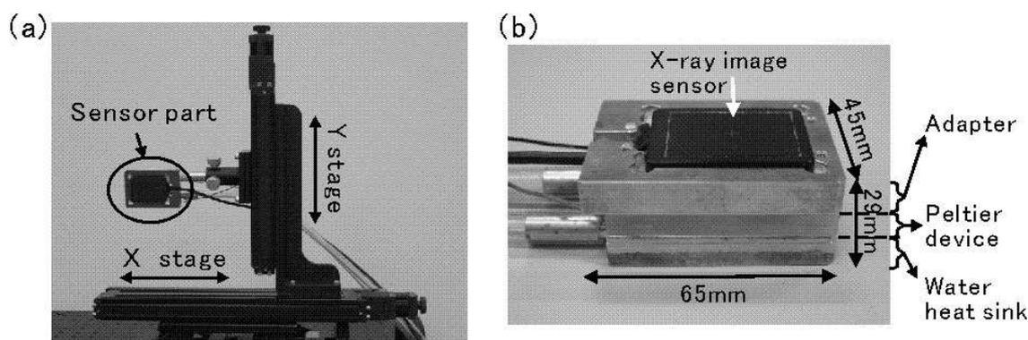
Fig. 3 (a) Prototype of x-ray imaging system applicable to a narrow space and (b) magnification of the sensor part.
