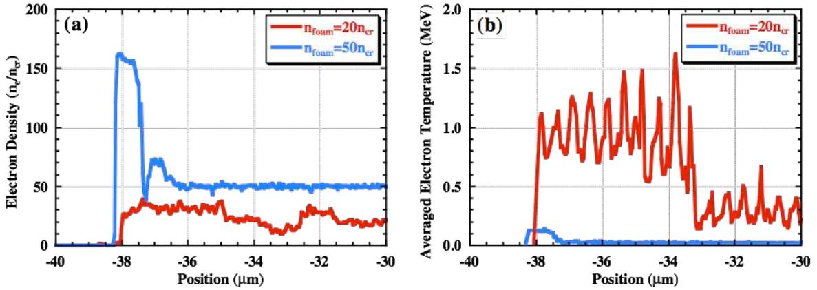
Fig.2. (a) Electron density and (b) averaged electron temperature profiles at  $t=1$  ps.
