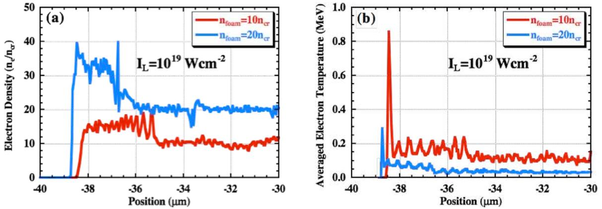
Fig.3. (a) Electron density and (b) averaged electron temperature profiles at  $t=1.5$  ps for  $I_L=10^{19}$   $Wcm^{-2}$ .
