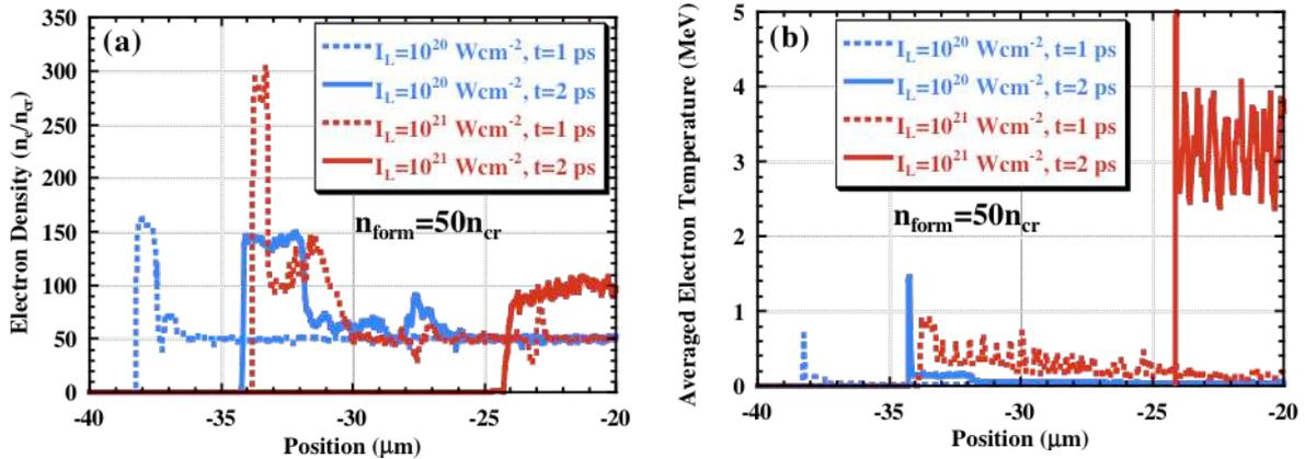
Fig.4. (a) Electron density and (b) averaged electron temperature profiles at  $t=1, 2$  ps for  $I_L=10^{20}, 10^{21}$   $Wcm^{-2}$ .
