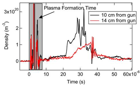
**Figure 2** Plasma density at different distances from the gun shows bubble propagation. Argon plasma data shown.
