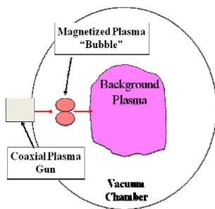
**Figure 1** Schematic layout of plasma bubble injection experiment.
