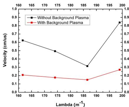
**Figure 3** Plasma bubble propagation behavior with and without background plasma. Lambda is a common coaxial gun operating parameter proportional to the ratio of gun current to bias flux.
