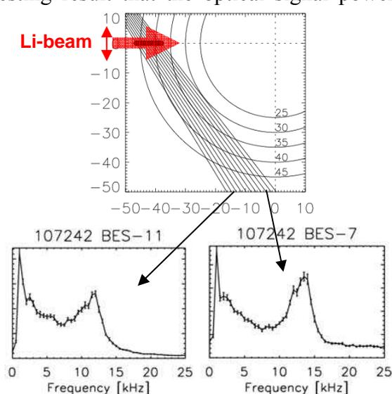
*Figure 3. GAM related peaks in background light fluctuation spectra and the measurement geometry.*
