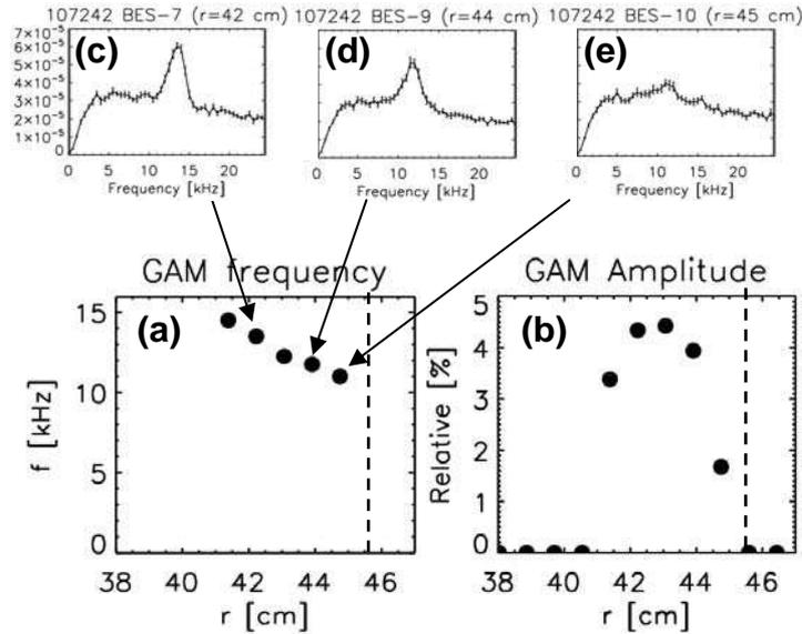
Figure 2. GAM measurements with the Li-beam diagnostic. (Shot 107242,  $I_p=350$ kA,  $B_t=2.25$ T,  $\langle n_e \rangle = 2 \cdot 10^{19} \text{m}^{-3}$ )
