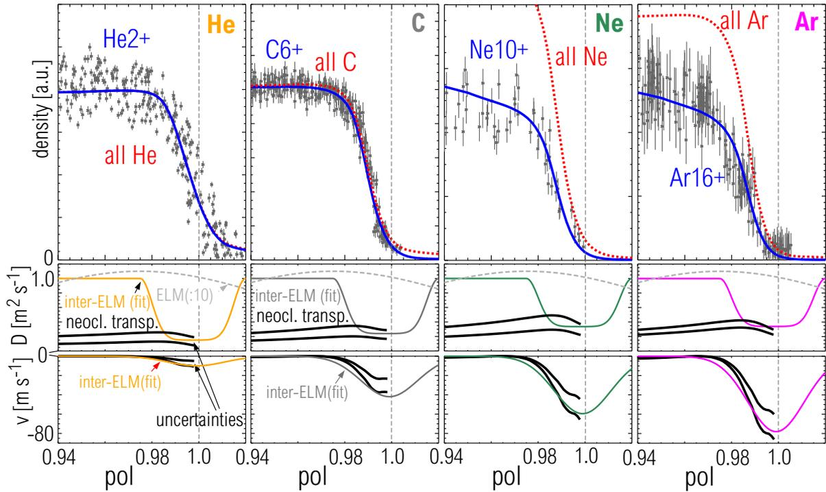
**Fig. 2:** Measured impurity density profiles along with the best fit of modelled profiles.
