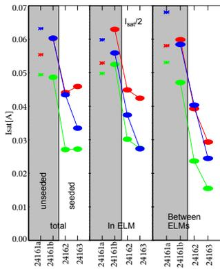
Figure 5: Mean  $I_{sat}$  for 3 filament probe tips in seeded (white background) and unseeded discharges. From left to right: total average, average during ELMs and average in between ELMs.
