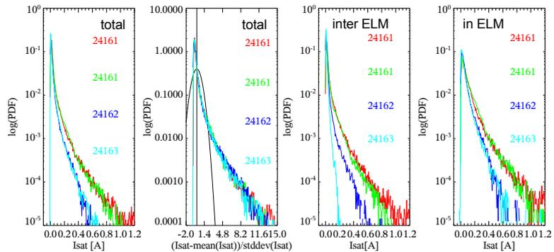
Figure 6: From left to right: PDF of  $I_{sat}$  at filament probe, normalized PDF, PDF of  $I_{sat}$  in between and in ELMs. All PDFs are shown for unseeded (red and green) and seeded (blue and cyan) cases.
