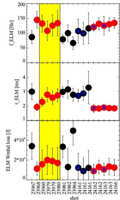
Figure 3: From top to bottom: ELM frequency, ELM duration, energy loss per ELM for the discharges in figure 1. Red corresponds to seeded, black to unseeded cases. Blue stars mark  $P_{NBI} = 5$  MW. The yellow background indicates seeding in the midplane.
