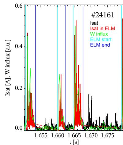
Figure 2: ELM filaments in  $I_{sat}$  at the outer midplane compared to the W influx in the divertor. The cyan and blue bars indicate ELM start and end times as determined from the W influx.
