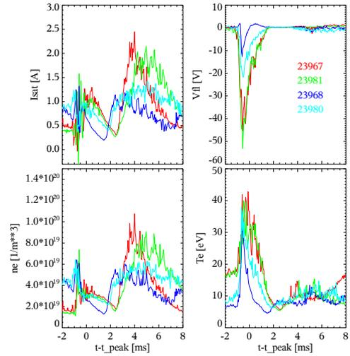
Figure 4: Time traces of  $I_{sat}$ ,  $V_{fil}$ ,  $n_e$  and  $T_e$  for a Langmuir probe in the divertor about 2.5 cm outside the separatrix.
