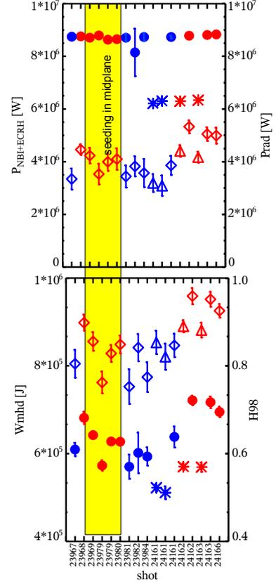
Figure 1: Top: Heating power (circles and stars), radiated power (diamonds and triangles), bottom: energy content (circles and stars) and H-factor 98Py2 (diamonds and triangles). Stars and triangles correspond to discharges with  $P_{NBI} = 5$  MW, circles and diamonds to  $P_{NBI} = 7.5$  MW. Red indicates seeded, blue unseeded discharges.
