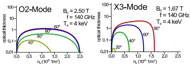
Figure 1: Angular dependence of the optical thicknesses of the O2- and X3-mode. [2, 3]
