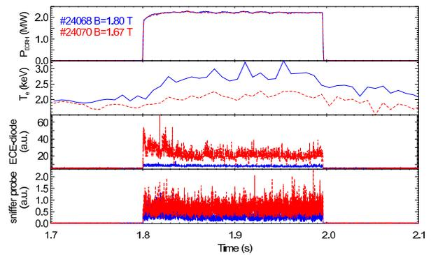
Figure 3: Discharges with X3-heating and  $B = 1.67 \text{ T}$  (red, dashed) and  $1.8 \text{ T}$  (blue). From top to bottom: ECRH power, electron temperature, ECE-diode and sniffer probe.
