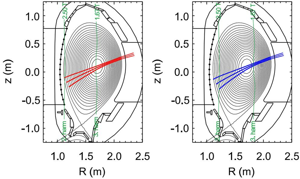
Figure 2: TORBEAM calculations for the X3-heating scenario at a magnetic field of 1.67 T (left, red) and 1.8 T (right, blue).
