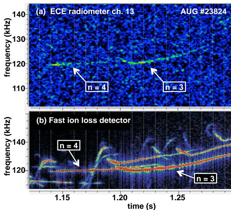
Figure 3. ECE and FILD data from a discharge with several TAEs, illustrating the possibility of spatially localizing particular modes. (a) A spectrogram of the ECE radiometer channel in which the peak amplitudes for two of the TAEs ( $n = 3$  and  $n = 4$ ) were detected. (b) The FILD spectrogram for the same time period, showing the fast ion losses from TAEs of many mode numbers—the two that were isolated in ECE are indicated.
