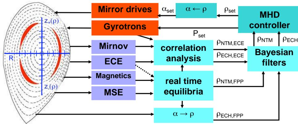
**Figure 1.** The real time NTM control loop. The NTM position is determined by the ECE-Mirnov correlation result mapped onto a real time equilibrium for flux coordinate  $\rho$  output. ECRH/ECCD mirror angles are updated, and modulated power deposition is located in ECE.
