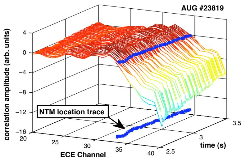
**Figure 2.** Tracking a  $3/2$  NTM via correlation of ECE and magnetic reference signals. A time series of correlation profiles is shown. Each profile is constructed by correlating all relevant radiometer channels with the single magnetic reference. The zero-crossing of each profile indicates the NTM center. The blue trace of zero-crossings is projected onto the ECE channel-time plane to illustrate the algorithm output.
