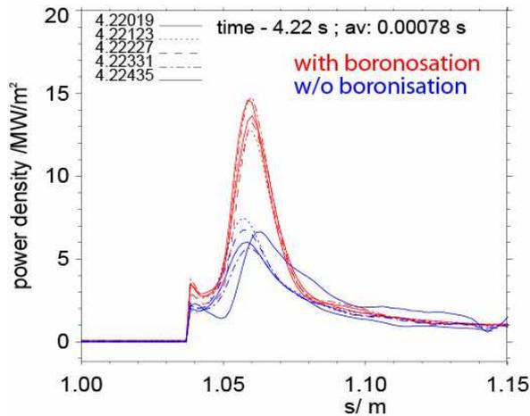
Fig. 3 Heat load in between ELMs to the outer strike line. The profiles are averaged over 4 time slices.
