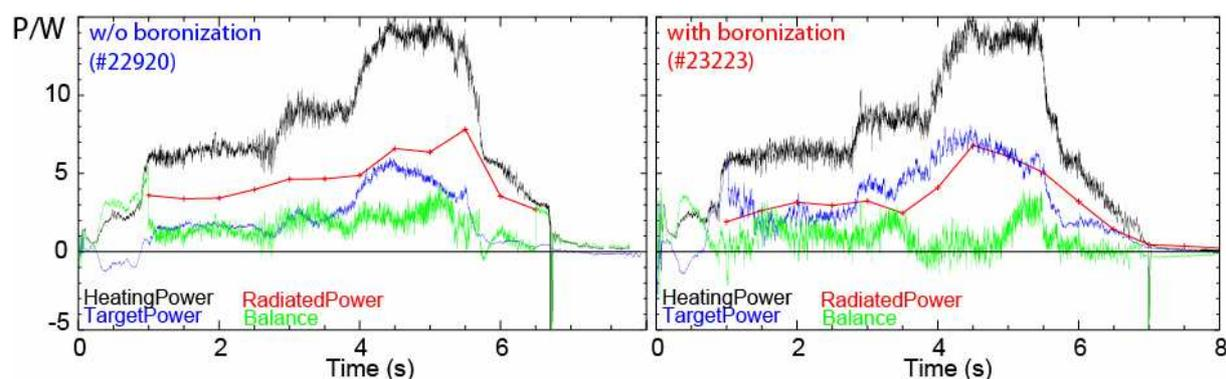
Fig. 2 Power balance for the discharge w/o and with boronization.
