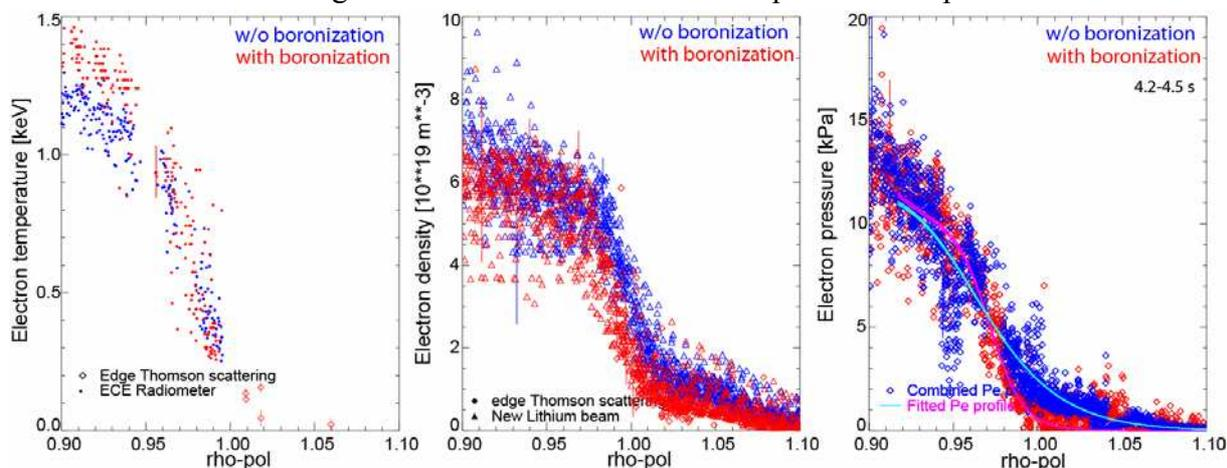
Fig. 5 Edge profiles of  $T_e$ ,  $n_e$  and the resulting electron pressure.
