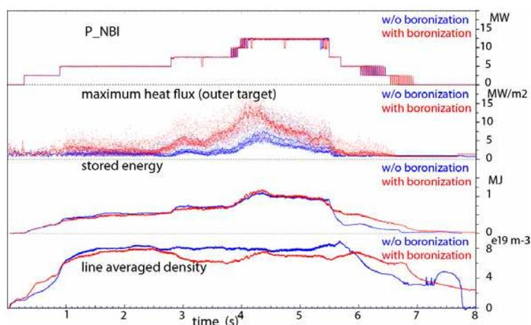
Fig. 1 Time traces for discharges before and after boronization.
