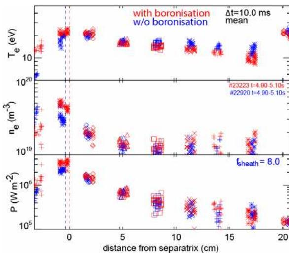
Fig. 4 Outer divertor parameters from Langmuir probes.
