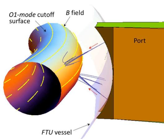
Fig.4: 3D poloidal view of FTU region where the new launcher will be installed. O1-mode cutoff layer and B field have been reconstructed using real high density plasma parameters of FTU. The paths of some rays, calculated using ECWGB ray tracing code, are also shown, showing the perfect poloidal and toroidal symmetry of the launcher (used as a launching system in the case considered in the figure).
