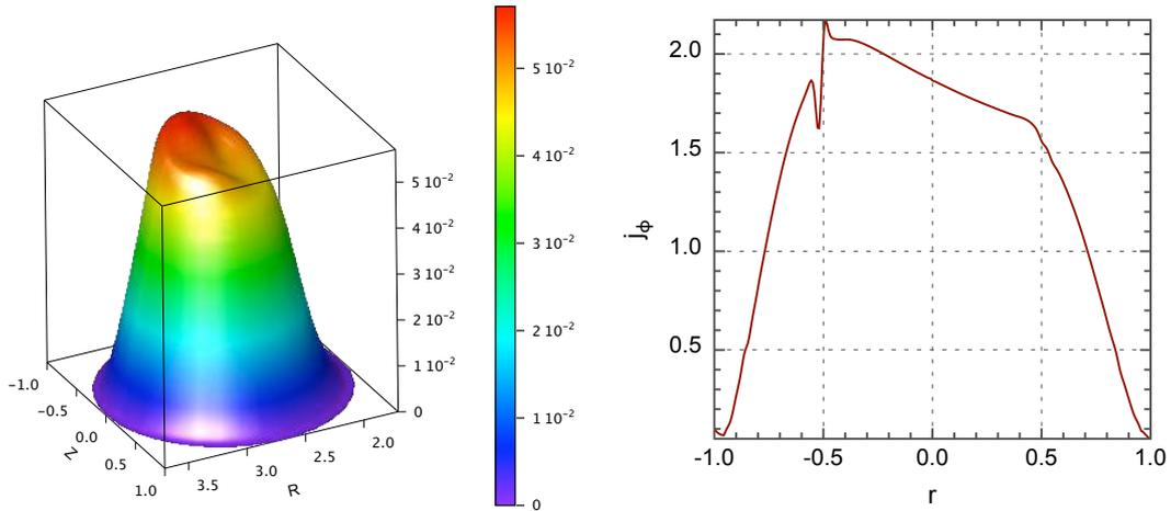
FIG. 4 – Left : 3-D pressure plot and right :  $j_\phi$  versus  $r$  in saturated regime for  $\beta_p = 0, 14$ ,  $\chi_\perp = 3.10^{-5}$ ,  $\chi_\parallel = 10$ .
