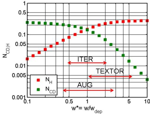
Figure 1: Geometrical efficiency for ECCD and ECRH (green and red squares, respectively), calculated at  $x_{dep} = 0$  with continuous power deposition. Red arrows refer to the typical range of a 3/2 island in AUG and ITER, and of a 2/1 island in TEXTOR.
