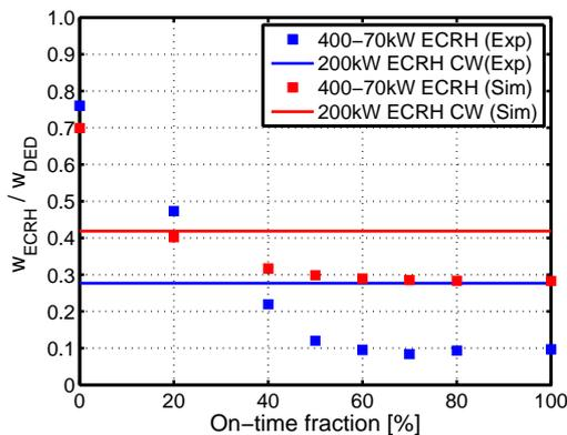
Figure 3: *Suppression of a 2/1 mode by modulated ECRH centered around the O-point as a function of the duty cycle of the ECRH high-power phase. Red markers refer to the numerical calculation while blue markers to experimental data. Solid lines refer to the continuous power deposition case. When the on-time fraction exceeds 60%, no further improvement on the stabilization is observed.*
