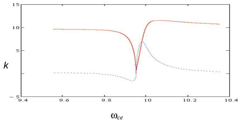
Fig.3 The real (full) and imaginary (dotted) parts of  $k$  when  $\omega=10+0.1287i$ . The real and imaginary parts both pass through zero when  $\omega_{ce}$  is a little below 10. The root with  $\text{Re}(k) \geq 0$  is plotted and there is of course a root with opposite sign.
