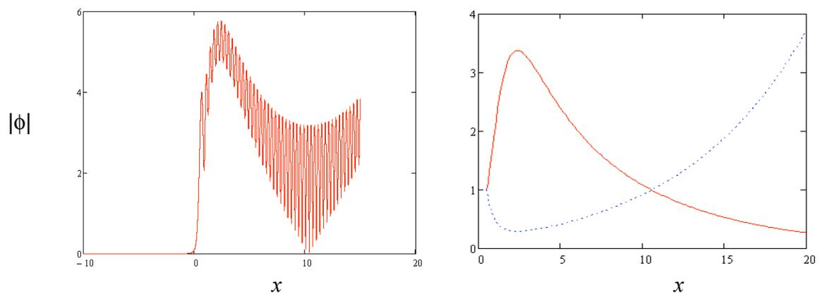
Fig.4 Numerical (left) and WKB (right) solutions for the wave amplitude. The outgoing wave in the right hand plot is the full line. In both cases outgoing and incoming waves have the same amplitude at around  $x=10$ .
