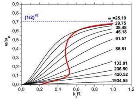
Fig. 5 Dispersion curves and phase diagram for  $l = 3$  wave mode
