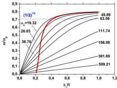
Fig. 4. Dispersion curves and phase diagram for azimuthally symmetric wave ( $l = 0$ )
