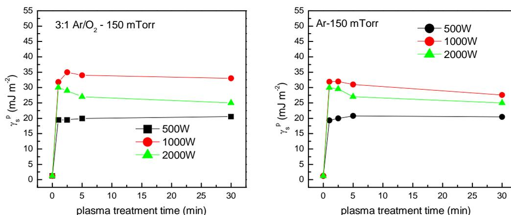
Fig. 1. The polar  $\gamma_s^p$  component of the free surface energy of PC treated in Ar and 3:1 Ar/O<sub>2</sub> plasma vs treatment time at indicated RF power.
