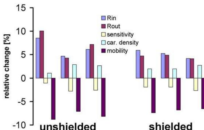
Figure 2: Comparison of relative change of physical parameters of the Hall sensors before and after the irradiation for shielded and unshielded samples.
