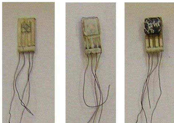
Figure 1: Left panel – bare Hall sensor before irradiation, middle panel – Hall sensor with sensing layer protected by *InSb/CdTe* glass shield, right panel – shielded Hall sensor after irradiation.
