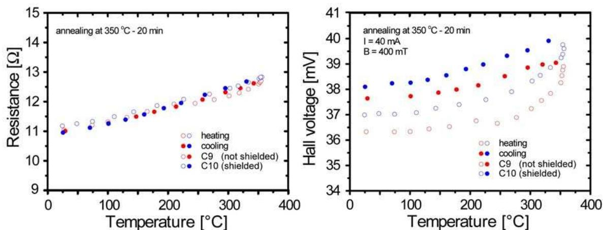
Figure 3: Impact of post irradiation annealing on sensors properties (left panel – Input resistance; right panel – Hall voltage for  $I_H=40$  mA and  $B=400$  mT).
