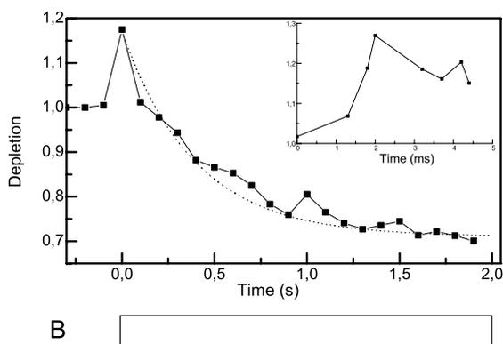
**Figure 3** Neutral depletion has a function of time during the ignition of the plasma, at 14 cm from the center of the plasma.
