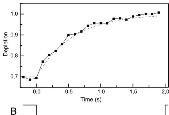
**Figure 2** Neutral depletion as a function of time during the afterglow at 14 cm from the center of the discharge.
