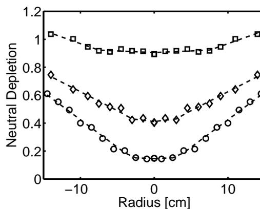
**Figure 1** Radial variation of the neutral gaz density in an helicon reactor for different magnetic field amplitude. This figure has been published in [6].
