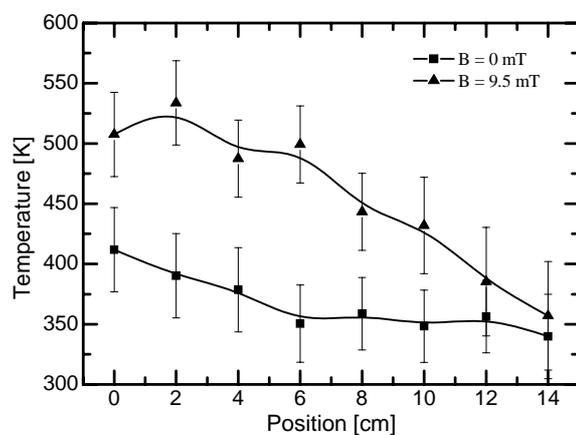
**Figure 4** Spatial variation of neutral temperature (Argon metastable) in the helicon reactor, with 500W, 10mTorr and different magnetic fields.
