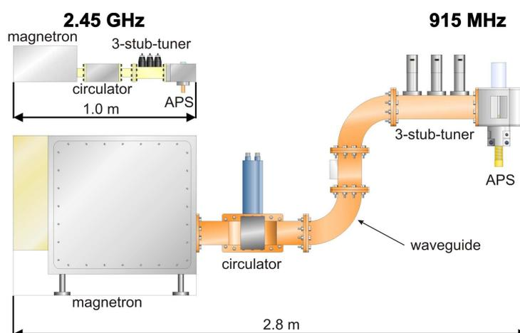
Figure 2: Schematic draw of the experimental set up and comparison between the 2.45 GHz and the 915 MHz atmospheric plasma source (APS).
