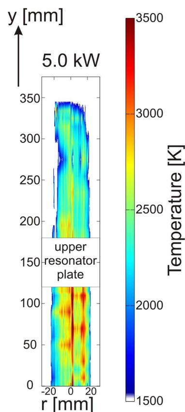
Figure 3: Temperature profile of the plasma at atmospheric pressure.
