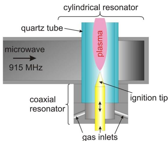
Figure 1: Schematic view of the resonator based plasma source.
