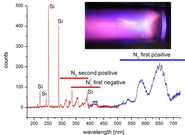
Figure 4: Overview spectra of a  $\text{N}_2$  plasma with silicon particulates and a photograph into the resonator.
