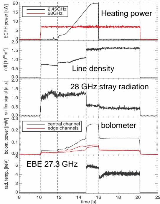
Figure 4: Time traces of a OXB-heated plasma operation. The transition takes place at 14.8 s.
