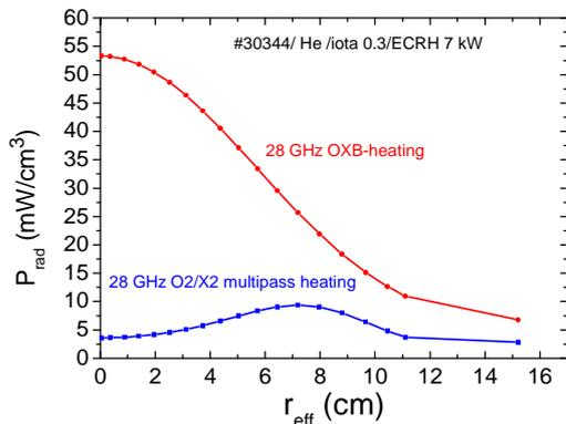
Figure 3: Radiation profile of over-dense EBW-heated plasma with central total single pass absorption in comparison with the profile of a low density plasma with multi-pass O2 heating. The profiles are reconstructed from the signals of a 12-channel bolometer camera.
