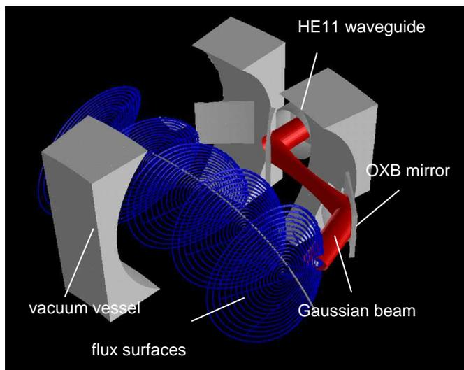
Figure 1: Quasi-optical transmission inside the WEGA vacuum vessel.
