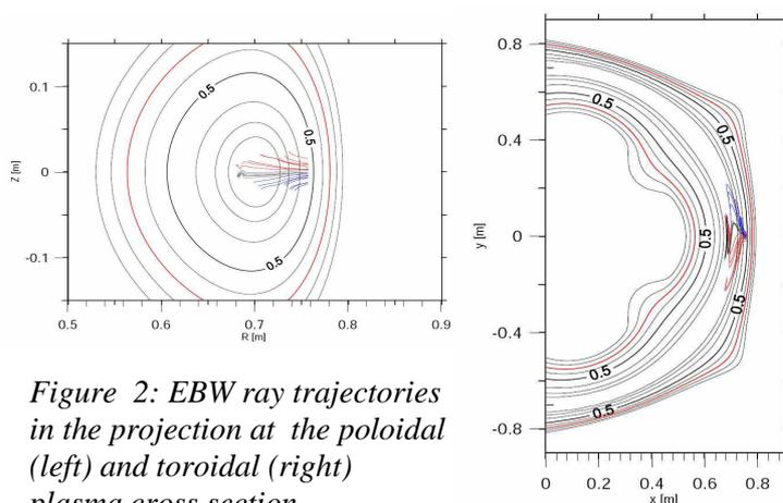
Figure 2: EBW ray trajectories in the projection at the poloidal (left) and toroidal (right) plasma cross section.
