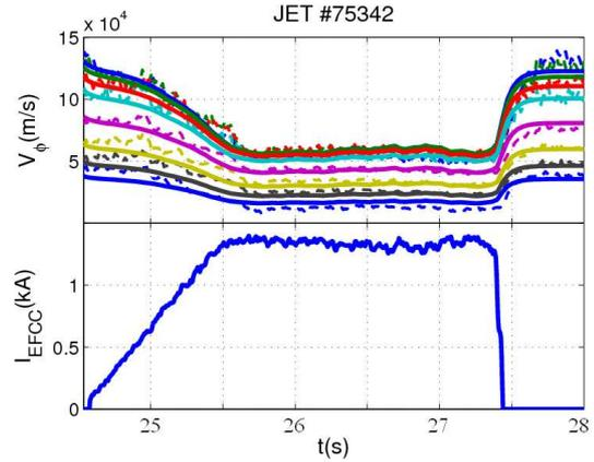
Figure 3. Comparison of the temporal evolution of the plasma velocity (top) from the experimental observation (star dashed line) and simulation (solid line). The bottom shows the time trace of the EFCC current.
