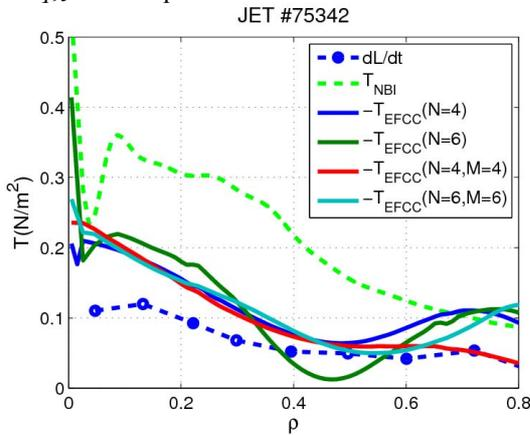
Figure 2. The obtained  $T_{EFCC}$  (solid line, times -1) profile by using the  $\chi_M$  and  $V_{inv}$  profiles fitted from different orders of polynomial base functions, the NBI torque (dashed line) and  $dL/dt$  (circles + dashed line) at the time just after the switch-off of the EFCC current.
