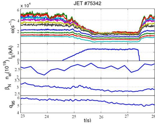
Figure 1. From top to bottom, the plasma angular rotation frequency at different radii, the EFCC current  $I_{EFCC}$ , the plasma density, normalized  $\beta$  and  $q_{95}$  for JET pulse 75342.
