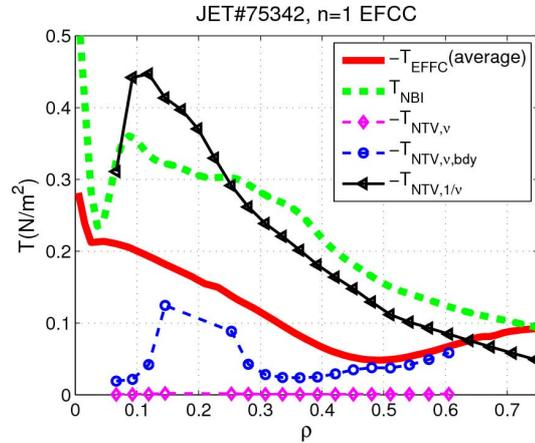
Figure 4. Comparison of the NTV torque (the triangles are the NTV torque in the  $1/\nu$  regime, the diamonds are that in the  $\nu$  regime, the circles are the boundary layer contribution in the  $\nu$  regime) with  $T_{EFCC}$  (solid line, averaged over the four profiles in Figure 2).
