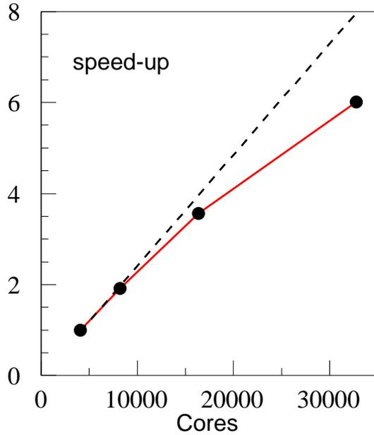
Figure 1: *Electrostatic ORB5: strong scaling. Relative speed-up from 4k to 32k cores for the Cyclone base case [4]; grid size: (128,512,256),  $3 \times 10^9$  markers. Simulations performed on BlueGene/P, in collaboration with RZG Garching.*
