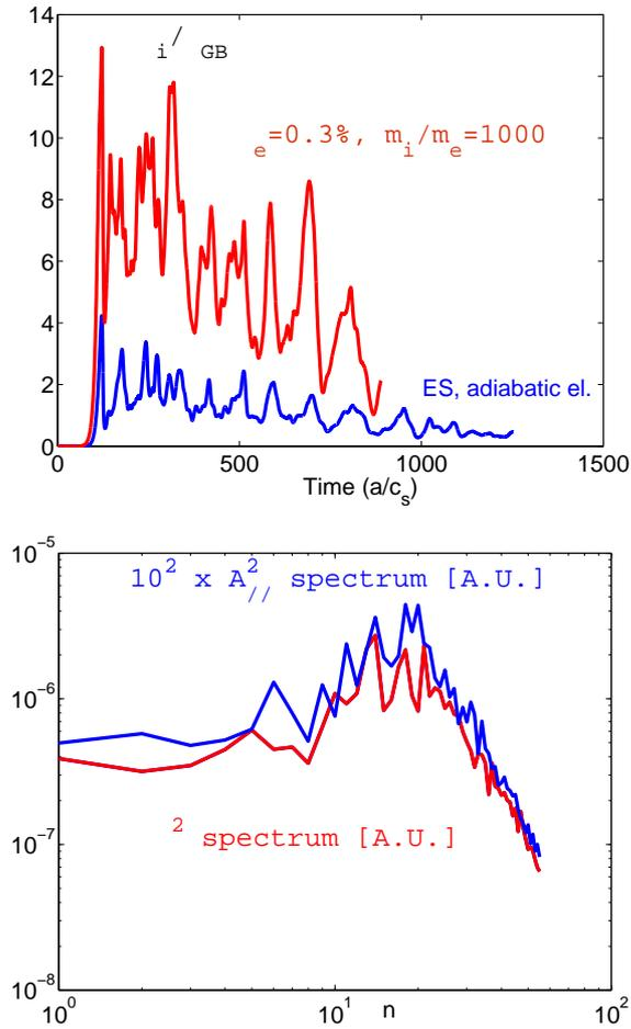
Figure 3: *Top*: time evolution of the ion thermal diffusivity for an electromagnetic  $\beta_e = 0.3\%$  EM simulation (red). *Bottom*: spectrum of the potential fields at  $t \simeq 800$   $[a/c_s]$ ;  $n$ , toroidal mode number.
