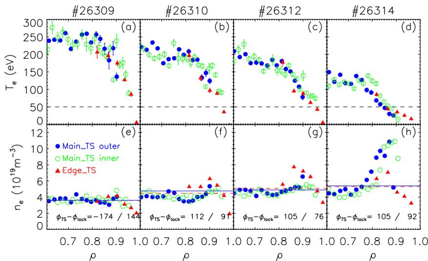
Figure 1: TS profiles of temperature (a)–(d) and density (e)–(h) for a series of discharges with increasing  $n/n_G$  (left to right,  $n/n_G = 0.28, 0.35, 0.44$  and 0.6). Dashed line in (a)–(d) marks  $T_e = 50$  eV.
