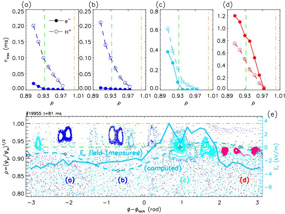
Figure 3: (a)–(d): Travel times as a function of  $\rho$  for particles deposited at  $\rho = 0.98$  and at toroidal angles corresponding to the labels (a)–(d) in frame (e); (e) Toroidal Poincaré plot with measured (solid) and computed (dashed) electric field.
