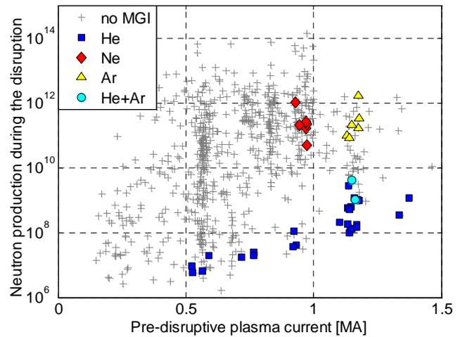
Fig. 1. Neutron production showing runaway amounts during Tore Supra disruptions. Background level is between  $10^6$  and  $10^8$ .
