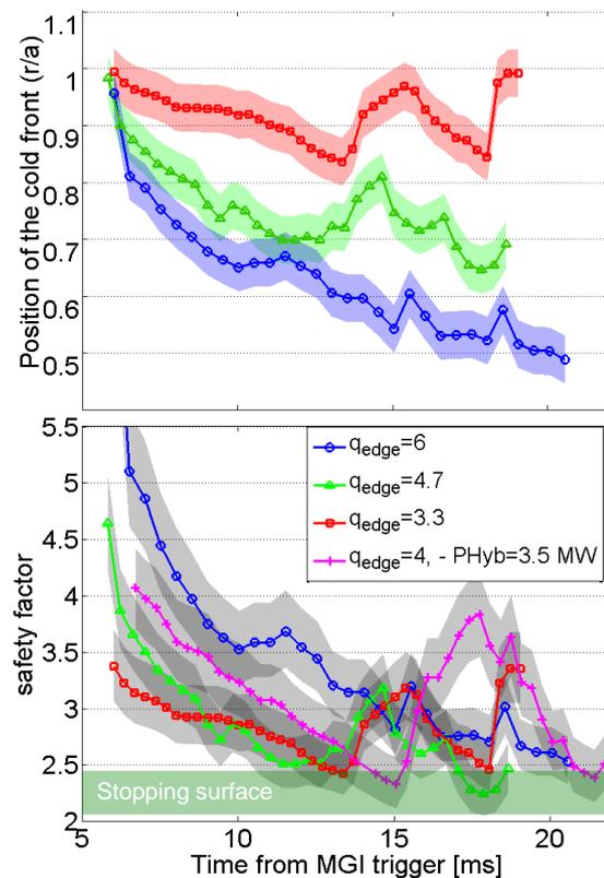
Fig. 4. Penetration of the cold front for different  $q$  profiles.  $25 \text{ Pa}\cdot\text{m}^3$  Helium injections. (a) penetration in normalized radius. (b) penetration in safety factor. Green zone on (b) shows the gas stopping area (between  $q=2$  and  $q=2.5$ )
