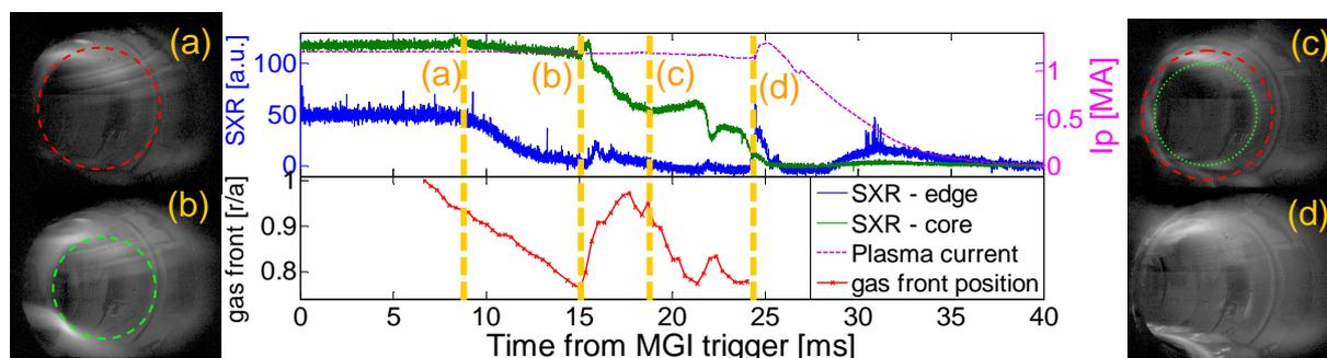
Fig 5. Disruption timeline : soft X-ray signal, plasma current and fast camera pictures at 4 times
