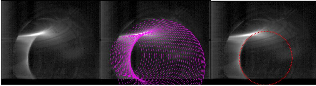
Fig 3. Shot 42047 - Position of the gas cold front (a) fast camera picture – (b) reconstructed flux surface ( $r = 55\text{cm}$ ) – (c) poloidal plane parallel to the endoscope lens
