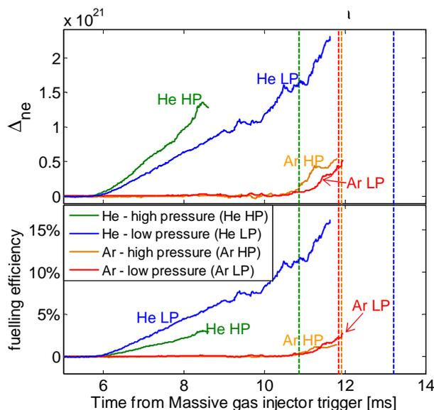
Fig 2. total amount of electrons added to the plasma by massive gas injections. (a): absolute value. (b): amount normalized to the number of particles injected. Vertical dashed lines are the thermal quench times. Helium reaches plasma edge at  $\sim 5.5$  ms, Argon at 7 ms
