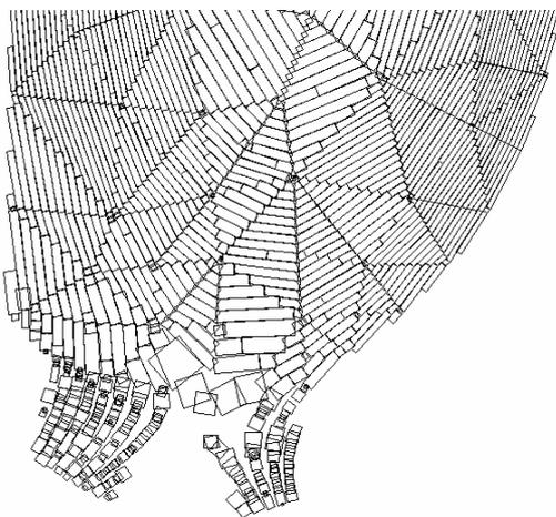
Fig. 2 Rectangular meshes of magnetic layers in TOKES
