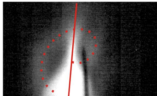
Figure 4: Image of plasma showing centreline of beam and spiral plasma structure. The dark object on the right of the beam is a Langmuir probe.
