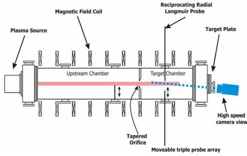
Fig 1: Schematic diagram of ULS linear plasma device showing location of main diagnostics used in this study.
