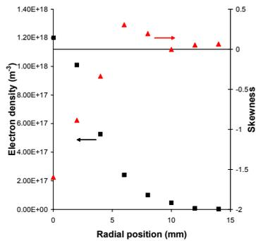
Figure 3: Radial Langmuir probe measurements of density, together with the skewness of the ion saturation PDFs, showing evidence for density deficits at the core plasma and blobs at the plasma edge.
