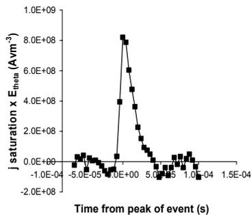
Figure 5: Product of ion saturation current density and azimuthal electric field at  $r=7.5\text{mm}$ , averaged over many intermittent events.
