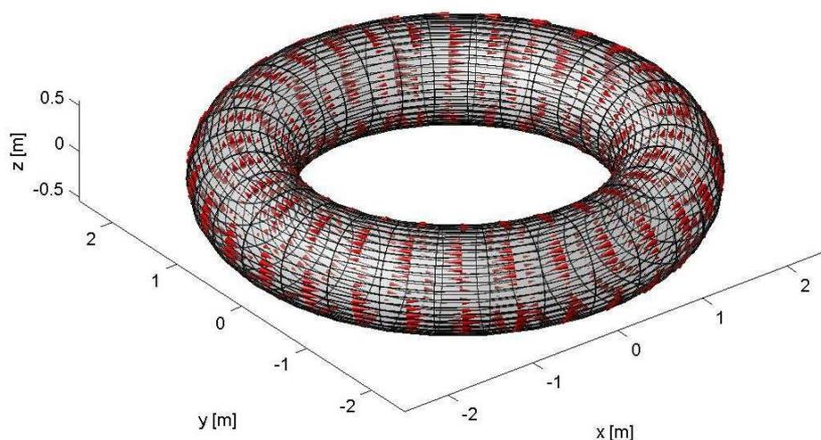
Figure 1. 3D view of the vessel mesh and current density (imaginary part)
