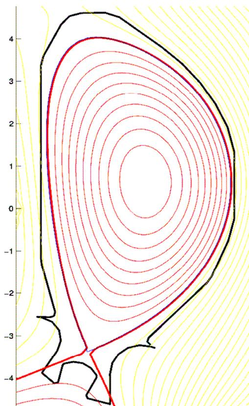
*EFIT\_ITM reconstruction (flux surfaces in red) of an ITER equilibrium generated with the DINA-CH code (boundary in blue) using the ITER machine geometry described in the ITM data structures.*
