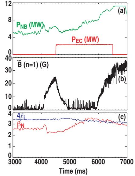
Fig. 3. Time history of (a) NBI and ECCD power, (b) rms amplitude of  $n=1$  mode, and (c) normalized beta and no-wall stability limit. In addition to the  $m/n=2/1$  NTM seen in (b), this hybrid scenario plasma also has a continuous and relatively benign  $m/n=3/2$  NTM.
