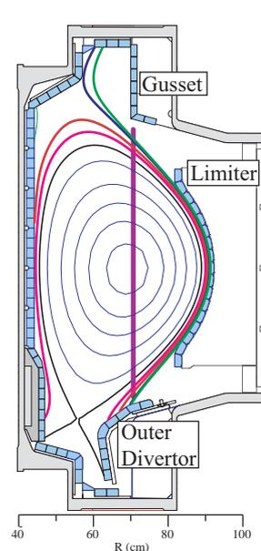
**Figure 2:** Schematic of flux surface reconstruction showing field line intersection with plasma facing surfaces.
