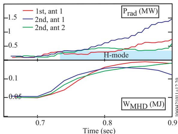
**Figure 3:** Second discharge following a boronization heated by second antenna has similar performance to the first discharge heated with antenna one following a boronization.
