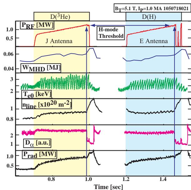
**Figure 1:** The plasma response in L-mode and the H-mode threshold are similar for D(3He) and D(H) minority heated discharges.
