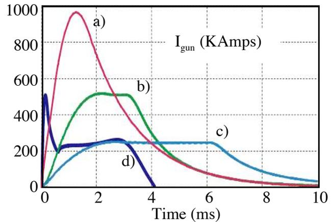
**Figure 1.** Predicted current waveforms from the new modular bank; a)  $\sim 1$  mega-ampere current pulse, b) extended formation current pulse, c) long current pulse and d) standard formation with sustainment pulse for comparison. Multiple current pulse not shown.
