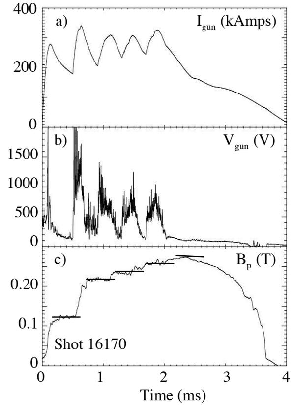
**Figure 3.** Time history of a multiple current pulse discharge; a) injected current with 5 pulses, b) gun voltage, and c) edge poloidal field showing stepwise increase in field. Note:  $I_{gun}$  and  $B_p$  y-axis scale different than in Fig. 2.
