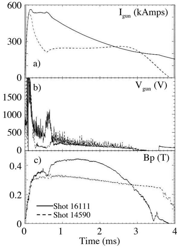
**Figure 2.** Time history of a long formation pulse discharge (solid) with standard fast formation followed by sustainment current pulse (dashed); a) injected current, b) gun voltage, and c) highest edge poloidal field measured on SSPX.
