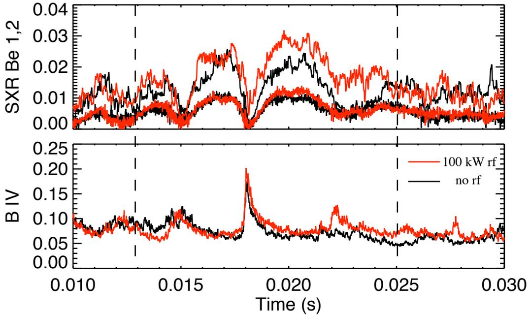
Figure 1: Measurable increase in soft x-ray emission during EBW injection (between vertical dashed lines). Emission is measured through two different thickness beryllium filters. There is a slight increase in boron IV emission during the same period, likely due to the boron-nitride construction of plasma facing components of the antenna.
