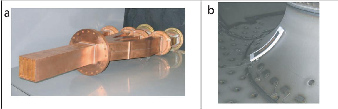
Figure 2: Left: photograph of four-guide EBW antenna, now installed on MST. Right: photograph of lower hybrid antenna installed in MST.
