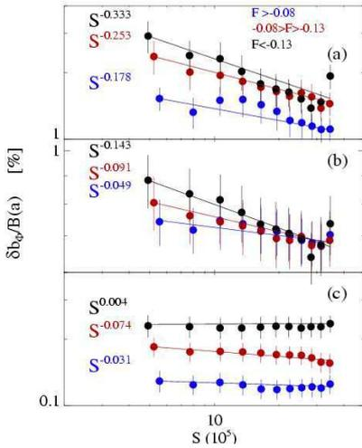
Fig. 5: Normalized RMS of the magnetic signals vs  $S$ : a)  $f < 10$ , b)  $10 < f < 60$ , c)  $f > 60$  kHz, for 3  $F$  values.
