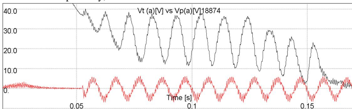
Figure 1: Time evolutions of toroidal (black) and poloidal (red) loop voltage oscillations during a vacuum test of OFCD operations at 100 Hz.
