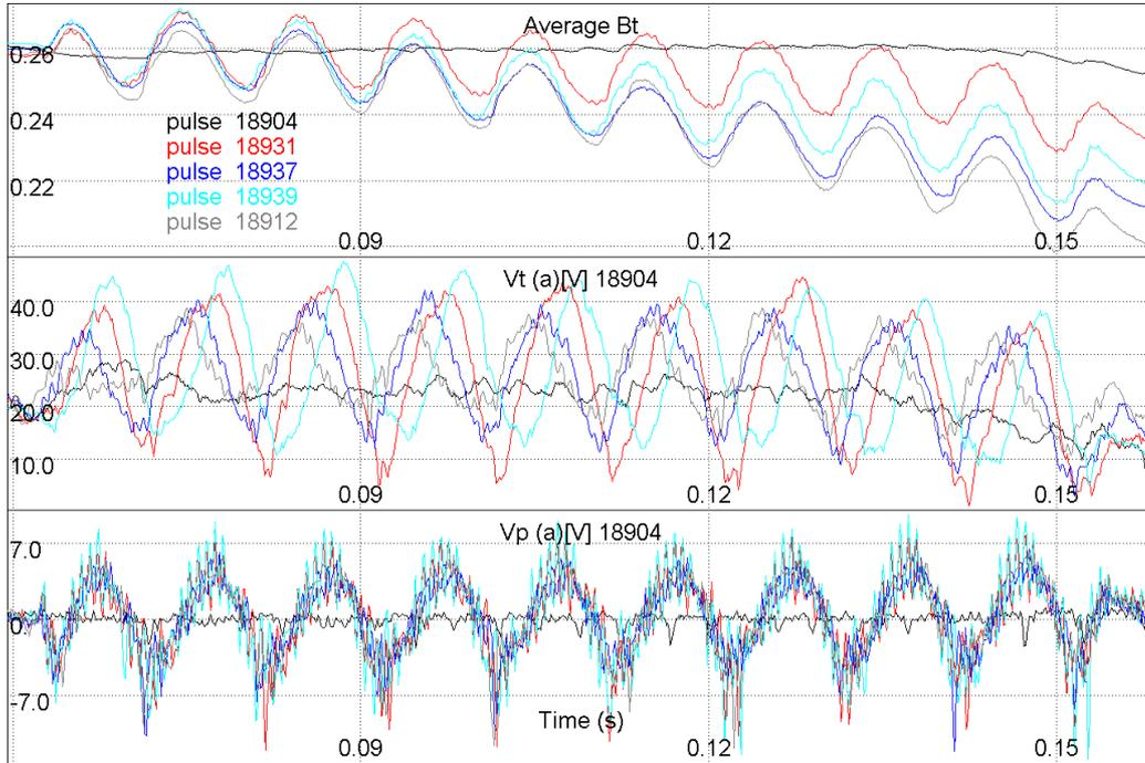
Figure 2: Example of phase scan for oscillations of about  $\pm 12$  V in the toroidal loop voltage (second window) and 6 V in the poloidal loop voltage (third window). Resulting toroidal flux is shown in the first window. Black (18904): reference; red (18931):  $\delta \approx 0$ ; blue (18937):  $\delta \approx \pi/4$ ; cyan (18939):  $\delta \approx -\pi/2$ ; grey (18912):  $\delta \approx \pi/2$ .
