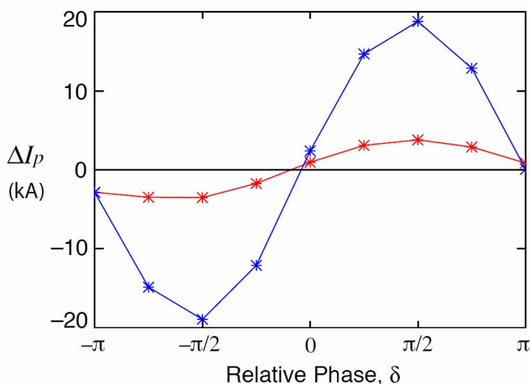
Figure 3: RFX-mod simulation of OFCD induced current versus relative phase for 2 cases. Red line: oscillation amplitudes as in the experiments described in the paper  $V_\phi = \pm 12V$  and  $V_\theta = \pm 6V$ ; blue line: possible result with values close to the maximum power available in the present system  $V_\phi = \pm 30V$  and  $V_\theta = \pm 15V$ .
