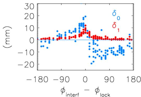
Figure 2:  $\delta_1$  and  $\delta_0$  component of the plasma column deformation
